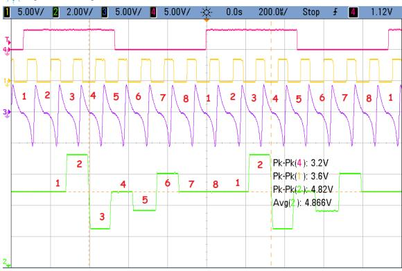
This mode of operation is independent of signal frequency. However, as speed/RPM ramps up or down, a steady deviation output will be produced. Once the RPM stabilizes, the delta-T analog output will return to center, with deviations indicated at the same scale factor of 5V/10%.
